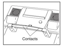
Next, **stand on the foot rails** and hold the metal contacts—**avoid moving your hands**. When your pulse is detected, the heart symbol in the right side of the display will appear, one or two dashes will appear, and then your heart rate will be shown. For the most accurate heart rate reading, continue to hold the contacts for about 15 seconds.
